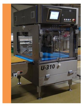
**Option** with two conveyor belts to push the product after cutting in distance. The length of the distance regulation with the speed from the second belt.
